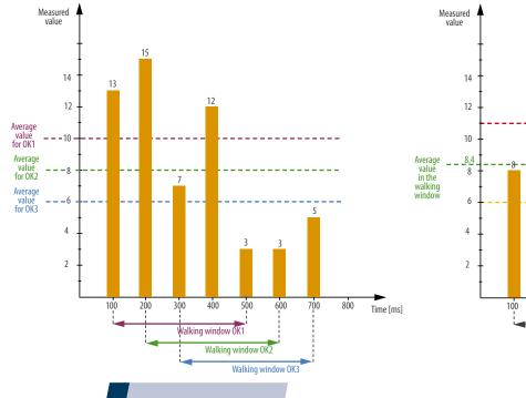
Programmed averaging time according to the walking window algorithm with a set averaging time. This function is useful for measuring high-dynamic signals.
