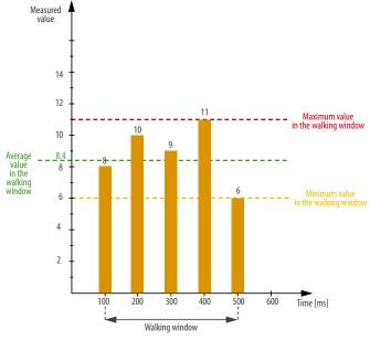
Ability to measure the average, minimum or maximum value when displaying the walking window.
