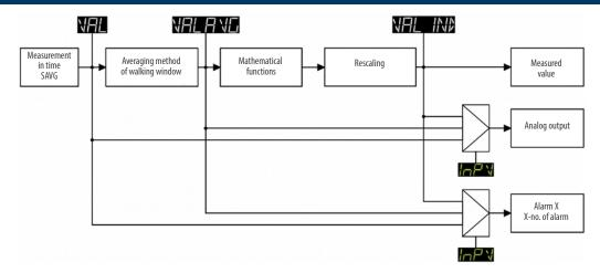
The measured value can be converted in series and the result can be displayed. After each conversion step, the signal can be used for retransmission on the analogue output or as an alarm source.
