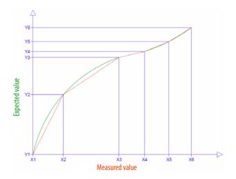
Conversion of the measured quantity based on 32-point individual characteristics. It allows for the mapping of signals from objects or sensors with non-linear characteristics.
