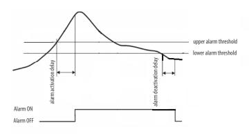
$t \ge$  time delay --> Alarm activeted For alarm operation both conditions (value and time delay) must be met
